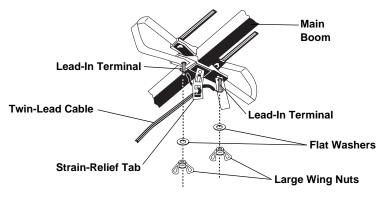
To connect flat, twin-lead cable to your antenna:
